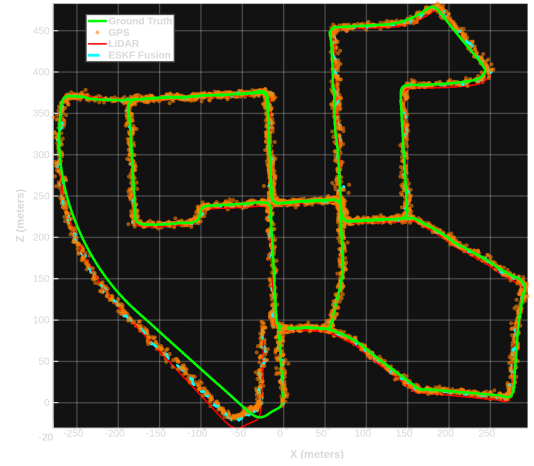
Figure 10: Trajectory deviation induced by the cross-space adversarial attack on A-LOAM with GNSS spoofing offset d = 0.2 m.
