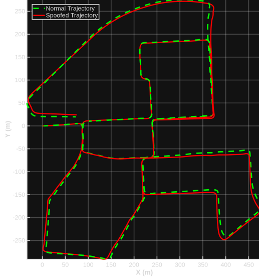
Figure 3: Accumulated Trajectory Drift due to LiDAR spoofing on A-LOAM.
